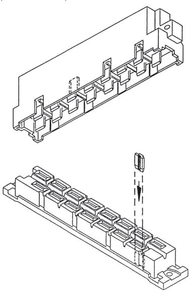
To avoid cross-plugging of adjacent connectors a coding system is required. Insert the code key 09 06 001 9918 into one of the keyways of the female connector as shown in the drawing. Break out the corresponding area of the male shroud. Connectors coded this way can only be applied in a minimum rack spacing of 20.32 mm.
