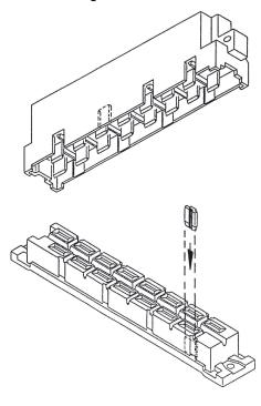
Insert the code key into one of the key ways of the female connector as shown in the drawing. Break out the corresponding area of the male shroud. Connectors coded this way can only be applied in a minimum rack spacing of 20.32 mm.
